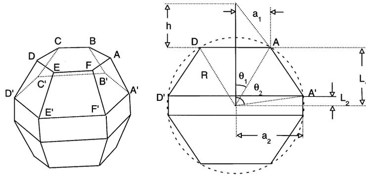
Fig. 4. The geometrical configuration of a droxtal.
