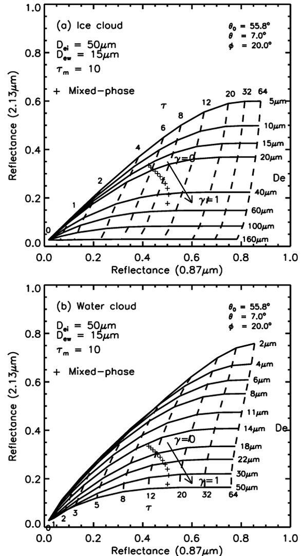
Fig. 2. Variation of the bidirectional reflectance for a mixed-phase cloud at 0.87 and 2.13  $\mu\text{m}$  with the ice fraction ( $\gamma$ ) superimposed on the theoretical  $\tau - D_e$  curves for the (a) ice cloud and (b) water cloud.  $\gamma$  varies from 0 to 1 as denoted by the (+) symbols.
