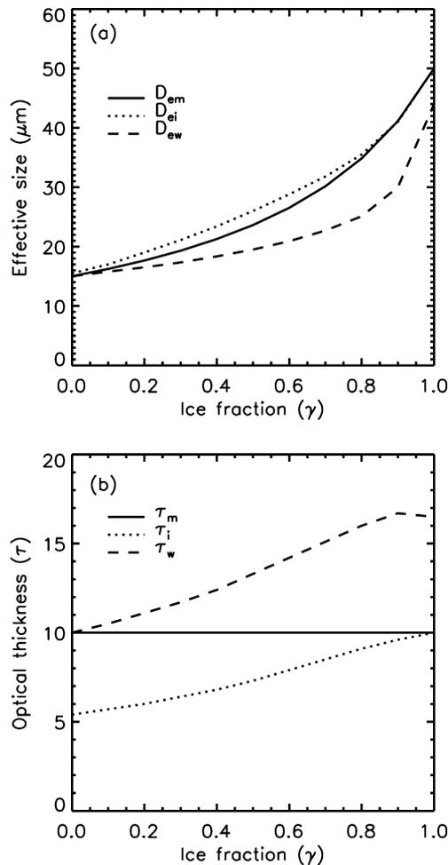
Fig. 3. Comparison of the (a) effective particle diameter and (b) optical thickness retrieved assuming a homogeneous ice and water cloud as a function of ice mass fraction ( $\gamma$ ). The true mixed-phase cloud parameters ( $\tau_m$ ,  $D_{em}$ ) are also shown.
