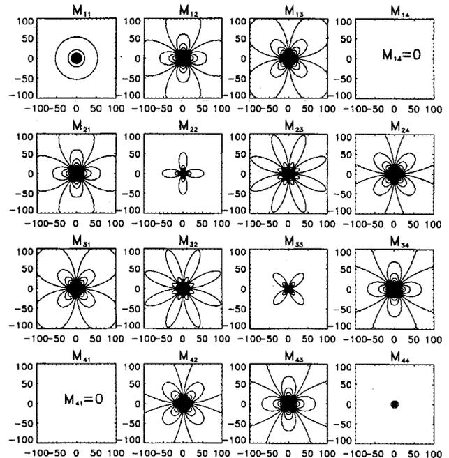
Fig. 7. Contours of the Mueller matrix for backscattering by ice spheres ( $R_{\text{eff}} = 100 \mu\text{m}$ ).
