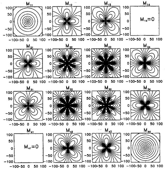
Fig. 4. Contours of the Mueller matrix for backscattering by randomly oriented hexagonal column ice crystals ( $2a/L = 100/600 \mu\text{m}$ ,  $R_{\text{eff}} = 113.5 \mu\text{m}$ ). The X and Y coordinates for each of the Mueller images indicate the positions of the pixels on the image plane (same as in Figs. 5–8).
