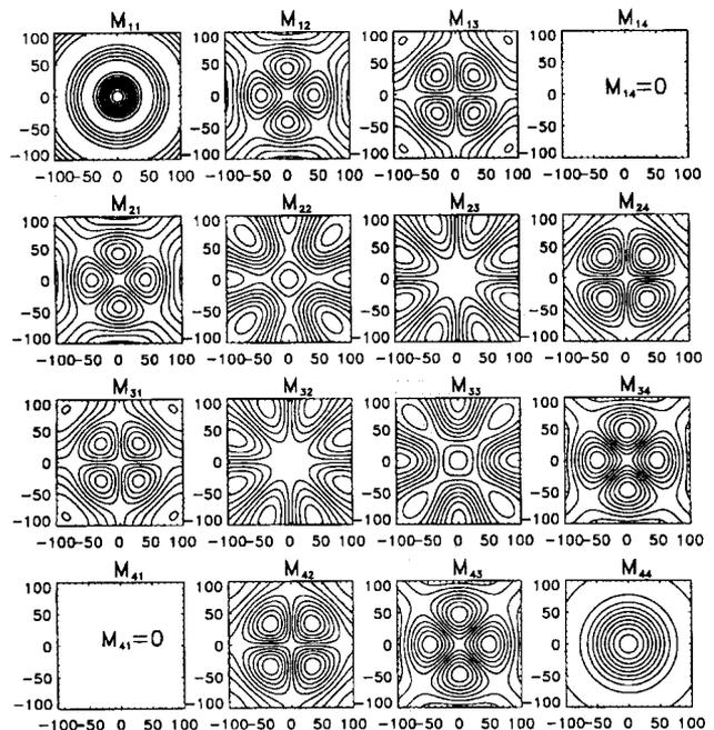
Fig. 8. Contours of the Mueller matrix for backscattering by spherical water droplets ( $R_{\text{eff}} = 4 \mu\text{m}$ ).
