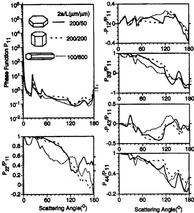
Fig. 2. Nonzero elements of the phase matrix for hexagonal ice crystals with three aspect ratios. Here,  $L$  and  $a$  are, respectively, the length and the radius of the cylinder circumscribing the ice crystal.
